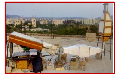
Solar air heater with thermal energy storage and food chamber
