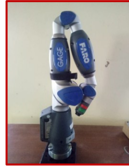
Portable Coordinate Measuring Machine (Faro Gage) with CAM2 Smart Inspect Pro
