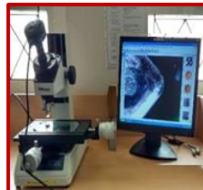
Tool Makers Microscope with camera & image analysis software
