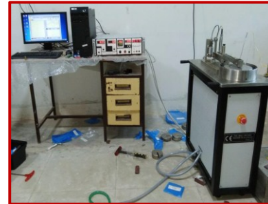
Pin/Ball on Disc Apparatus for Measurement of Friction & Wear by varying Temperature, Sliding Speed & Load
